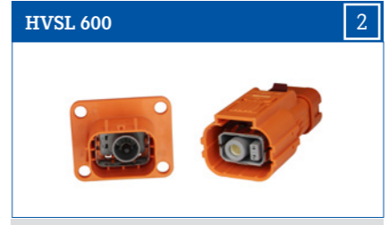
HVSL600 is a single pin connector, which provides a rated current of 120A and a 25mm² crimping cable. It can be used with multi-core or single-wire. An integrated internal HVIL with multiple routing options offers a package size optimization and flexibility.
