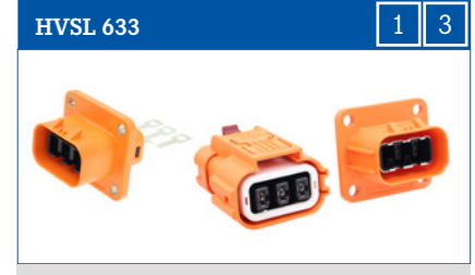
HVSL633 is a 3 positions connector, which offers a range of current from 23A to 40A and a 4 to 6mm² crimping. It was specially designed for DC-DC, air-conditioner and other EV equipment and devices.
