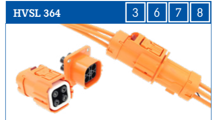
HVSL364: 4 pos. / up to 80A / 2.5 to 16mm² (shielded wire) HVSL364 was specially designed for DC-DC, air-conditioner, and other EV equipment and devices.
