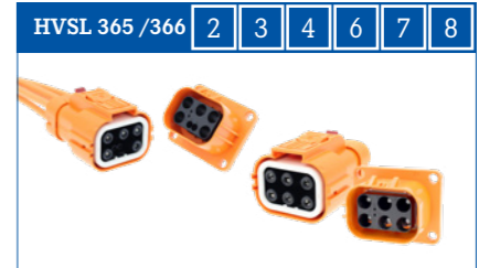
HVSL365 & HVSL366: 5 to 6 pos. / up to 40A / 4 to 6mm² (shielded wire) HVSL365 & HVSL366 were specially designed for DC-DC, air-conditioner, and other EV equipment and devices.
