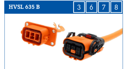
HVSL635B: 4 to 5 pos. / up to 40A / 2.5 to 6mm² (shielded wire) HVSL635B was specially designed for DC-DC, air-conditioner, and other EV equipment and devices.
