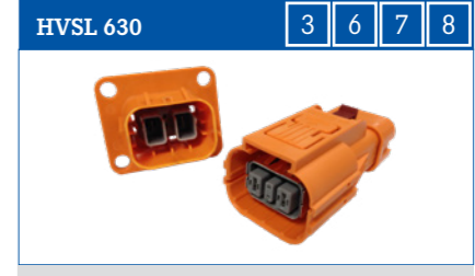
HVSL630 is a 2 positions connector, which offers a range of current from 23A to 40A and a 4 to 6mm² crimping. It was specially designed for DC-DC, air-conditioner and other EV equipment and devices.
