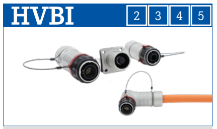
HVBI is an enhanced version of HV series connectors. This second generation of products offers an interlock system and high voltage. Rated current: 250A Max / rated voltage: 1000V DC / wire range: 16 to 70mm²
