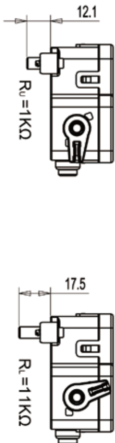
Emergency unlocking of the 12V locking actuator Schematic diagram
